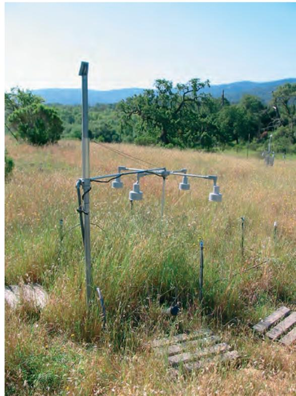
Fig. 3.5. An experimental plot in the Jasper Ridge Global Change Experiment. Four infrared heat lamps suspended over the 2-m diameter plot increase the canopy temperature by ~1 °C. Pure CO<sub>2</sub> is released from a circle of tubing surrounding the plot, enriching the CO<sub>2</sub> concentration in the air by about 300 ppm. Subplots comprise different combinations of precipitation and N deposition
